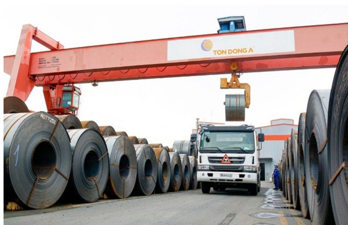
Figure 17: Hot-rolled steel (HRC) before being sent to the pickling line (in the galvanized steel plant).
