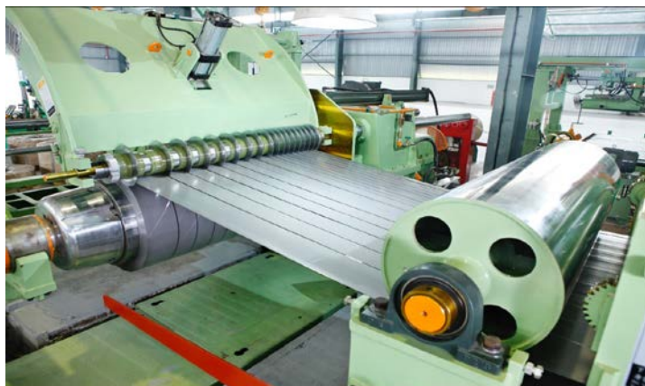
Figure 14: SMC's slitting and cutting lines in the coil processing segment
